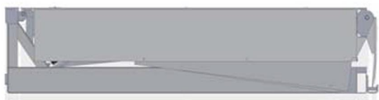
7. Final closed position of the leveler. Ready for the next operation.
