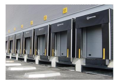
Red Steel Retractable Dock Shelter consists of a perimeter structure with a set of canvases attached to it. These canvases adjust to fit the body of the trailer. The structure is retractable so that, in the event of an impact, the shelter will return to its original position.
